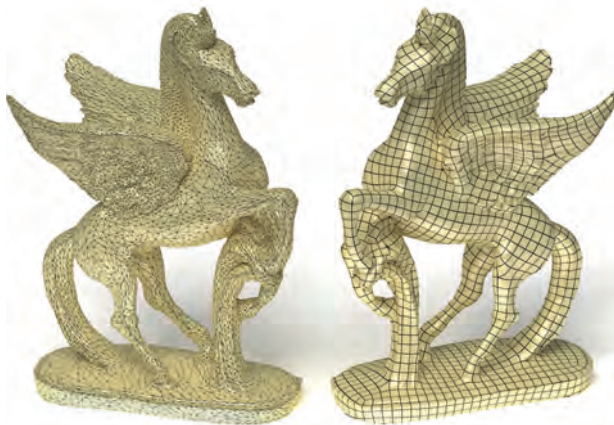
Figure 1. Automatic conversion of a triangle mesh (left) to a highly structured quadrilateral mesh (right)
